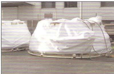
A tight, heated seal is not necessary for safe and effective long-term protection
